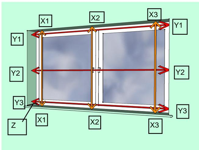
3. Measure the left drop Y1, the center drop Y2, and Y3 the right hand drop.
