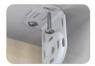
Insert two screws and tighten. Using the front and back slots allows for sideways adjustment of the of the bracket before completely tightening.
